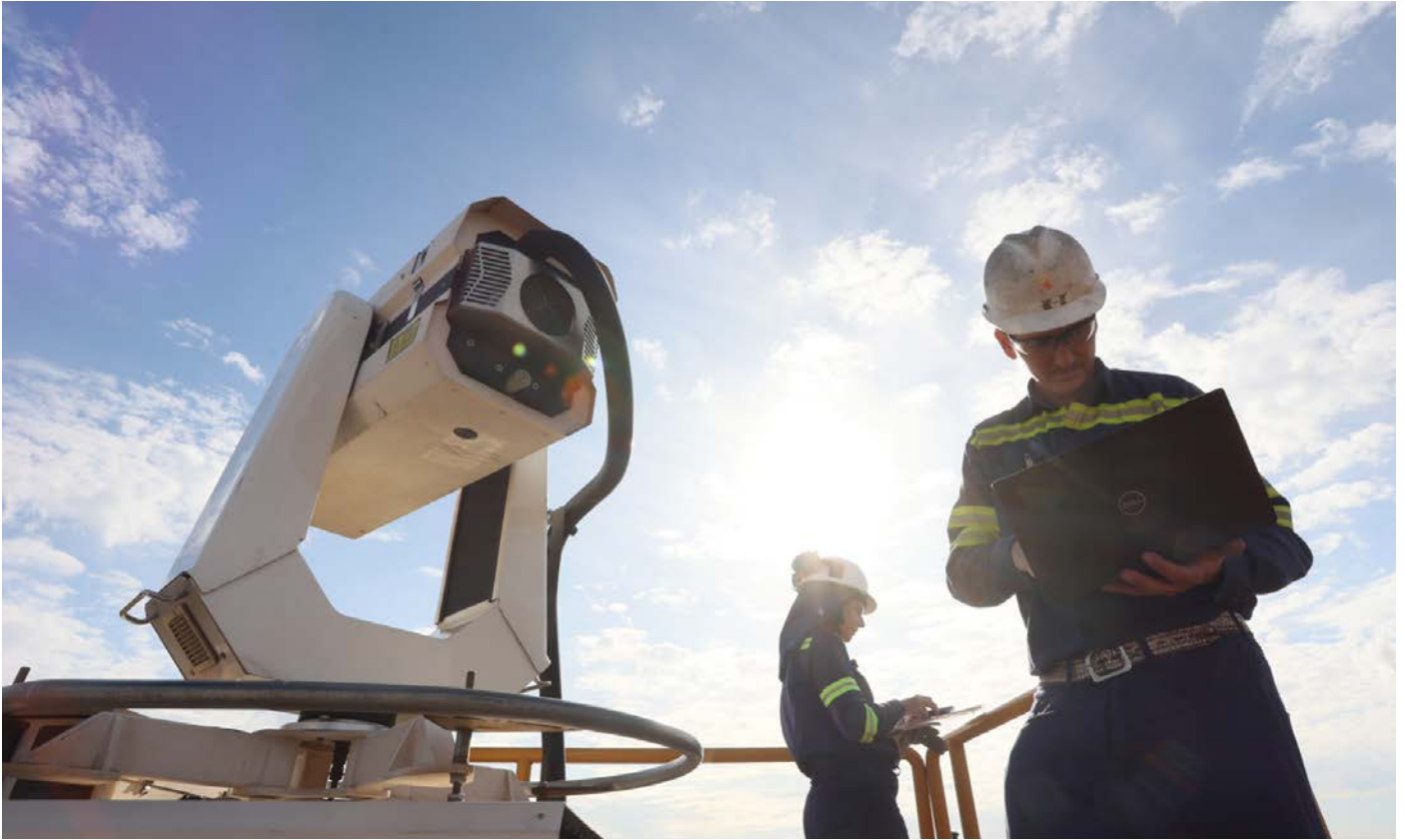
LiDAR (Light Detection and Ranging) technology. Currently undergoing testing at Ternium's San Nicolás unit in Argentina and the Rio de Janeiro unit in Brazil.
